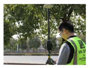
The G200 is a cost-effective GNSS receiver that provides centimeter accuracy positioning to connected mobile devices for RTK field surveying.
