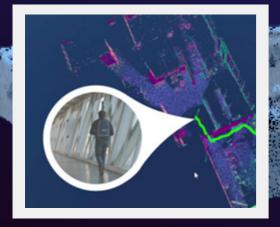
While walking, HERON® captures the reality around you, every five meters the 3D map is subdivided in block of scans. This group of points will be automatically connected consequentially.
