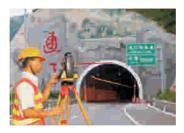
Tunnel Measurement Be able to observe measuring point without prisms. Pointlayout becomes easier
